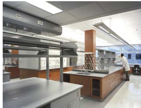
To create a light and open feel, Merck's chemistry labs include design elements such as exterior windows, flexible casework, and clear glass drying racks located above the sinks. (Photo courtesy of Kling, Paul Warchol Photography.)
